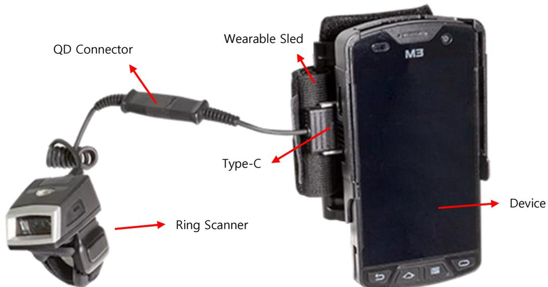
2: After connecting the wearable sled to the scanner, press the right button of the scanner to emit the scanner startup sound.
